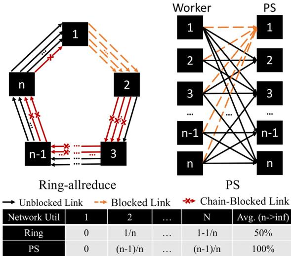
Figure 2: Ring allreduce suffers from chain blocking
